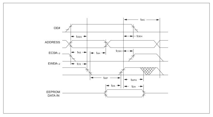
FIGURE 8 – EEPROM WRITE WAVEFORMS ECS# CONTROLLED
