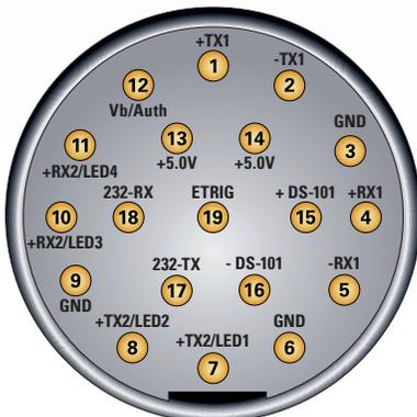
Pinout on 19 pin Receptacle
