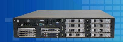
A part of the *EnterpriseSeries*", Mercury's RES-XR5 2U Server employs E5-2600 v3/v4 series Intel® Xeon® processors to accelerate compute intensive workloads for applications such as signal intelligence, cryptography, AI, sensor fusion, analytics, communications, and audio/video processing.
